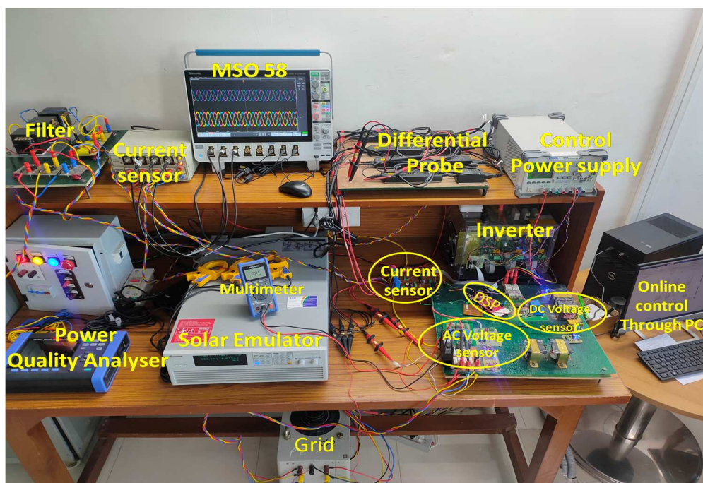
Figure 2.14: The hardware prototype developed in lab for experimental validation
