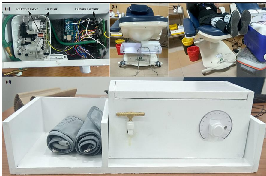
Figure.8.1 (a) Electronic components used in device, (b) Placement of device in Blood donor chair, (c) Device demonstration, (d) Final look of the device.
