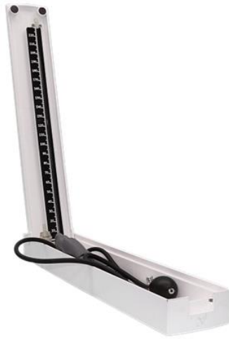
Figure.4.7. 3D manufactured full device end to end, enclosure box was manufactured by FDM method.
