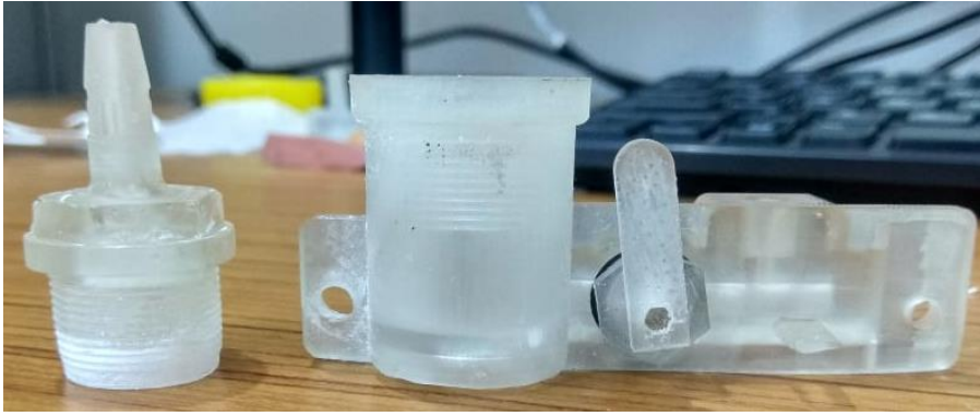
Figure.4.9 Final 3D manufactured part through SLA method.
