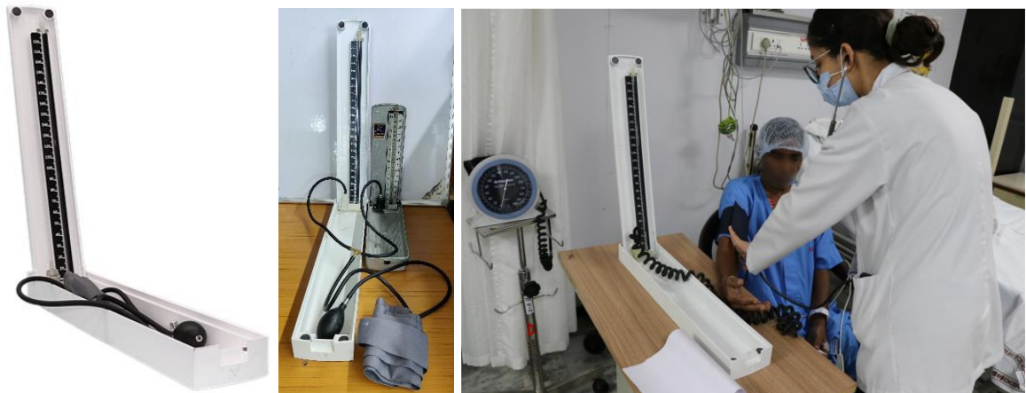
Figure. 5.1: (a) Complete alpha-prototype of Merkfree, (b) Technical comparison of Merkfree against MS through a T-connector joint. (c) Merkfree undergoing clinical trial at DMC&H Ludhiana.
