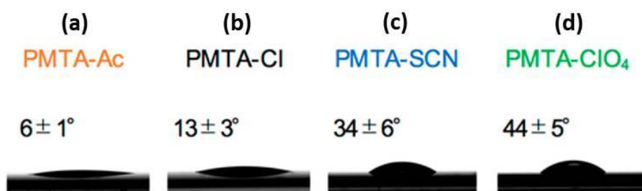
Figure 1.7 Side view of a water droplet on (a) PMTA-Ac, (b) PMTA-Cl, (c) PMTA-SCN, and (d) PMTA-ClO 4 . The averaged static contact angles are depicted in the images. Reprinted from Ind. Eng. Chem. Res. 2018, 57, 15, 5268-5275. Copyright 2018 American Chemical Society. 110
