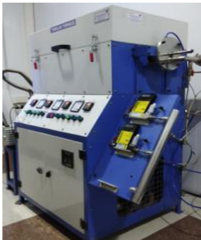
Figure AI.2 Atmospheric pressure chemical vapor deposition (APCVD) used to deposit MoS 2 flakes.
