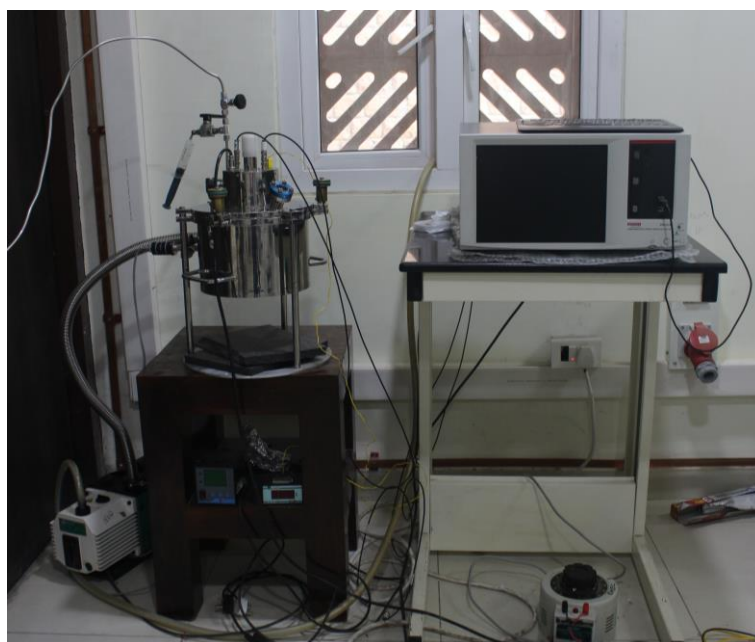
Figure AI.4 Gas sensing setup used to characterize MoS 2 -based gas sensors.
