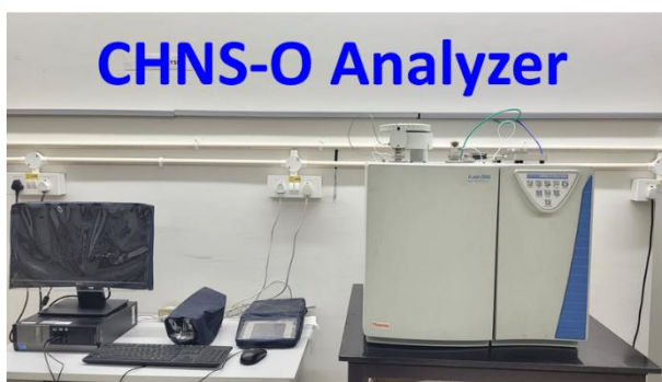
Figure 2-2. Image showing the CHNS-O elemental analyzer by Thermo Scientific used for CHNS-O measurements.
