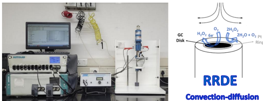
Figure 2-6. (a) Image representing the RRDE setup connected to Autolab 302 N potentiostat during ORR measurement under hydrodynamic conditions controlled by Pine rotator and (b) schematic representation of RRDE mechanism over rotating-ring disc electrode during ORR.
