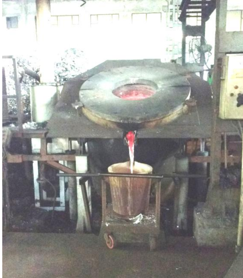
Figure 4.3 a hydraulically tilting furnace system feeding melted aluminium into a 100kg ladle at Prakash Alloy Udhyog in Jagadhari, Haryana, India.
