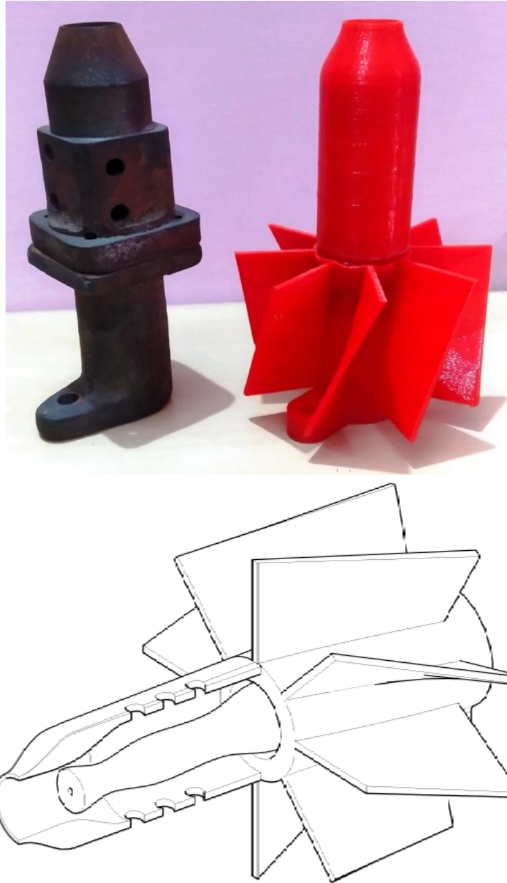
Figure 3.11 illustrates air swirl generators along with an image of the vane angle and air swirled.
