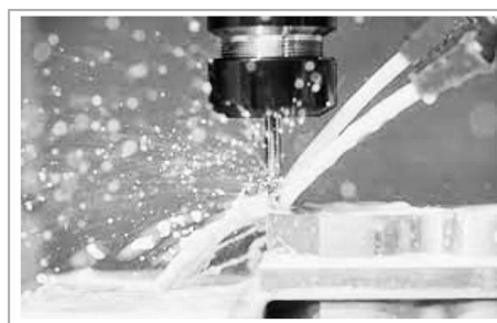
Figure 3.14 Schematic of conventional wet cooling approach used during machining
