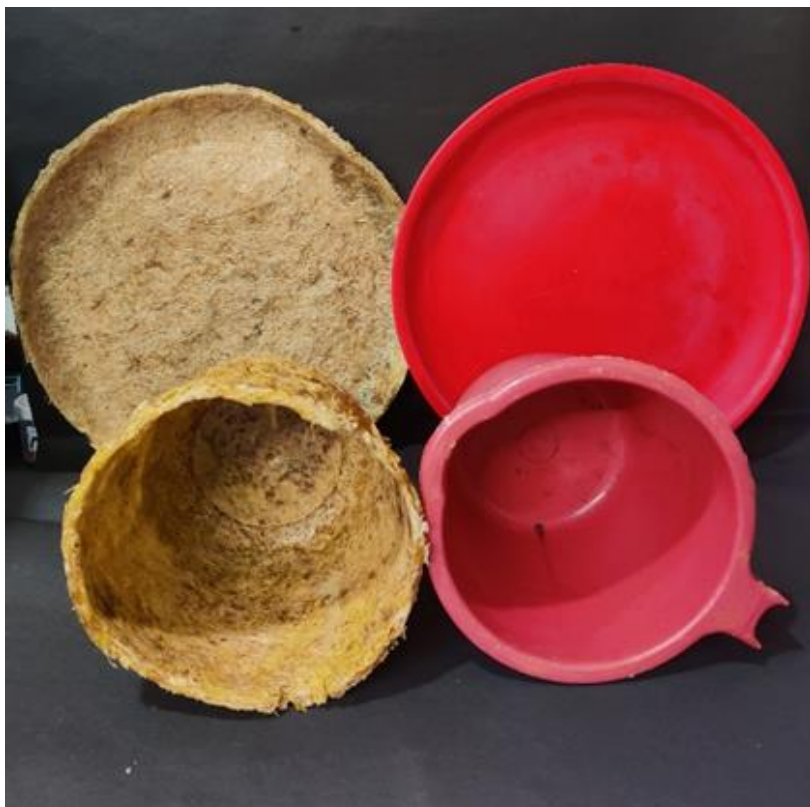
Figure 5.1. Plate and pot developed using treated waste Kibisu silk-wheat gluten composite sheets representing the feasibility of preparing various biodegradable products.
