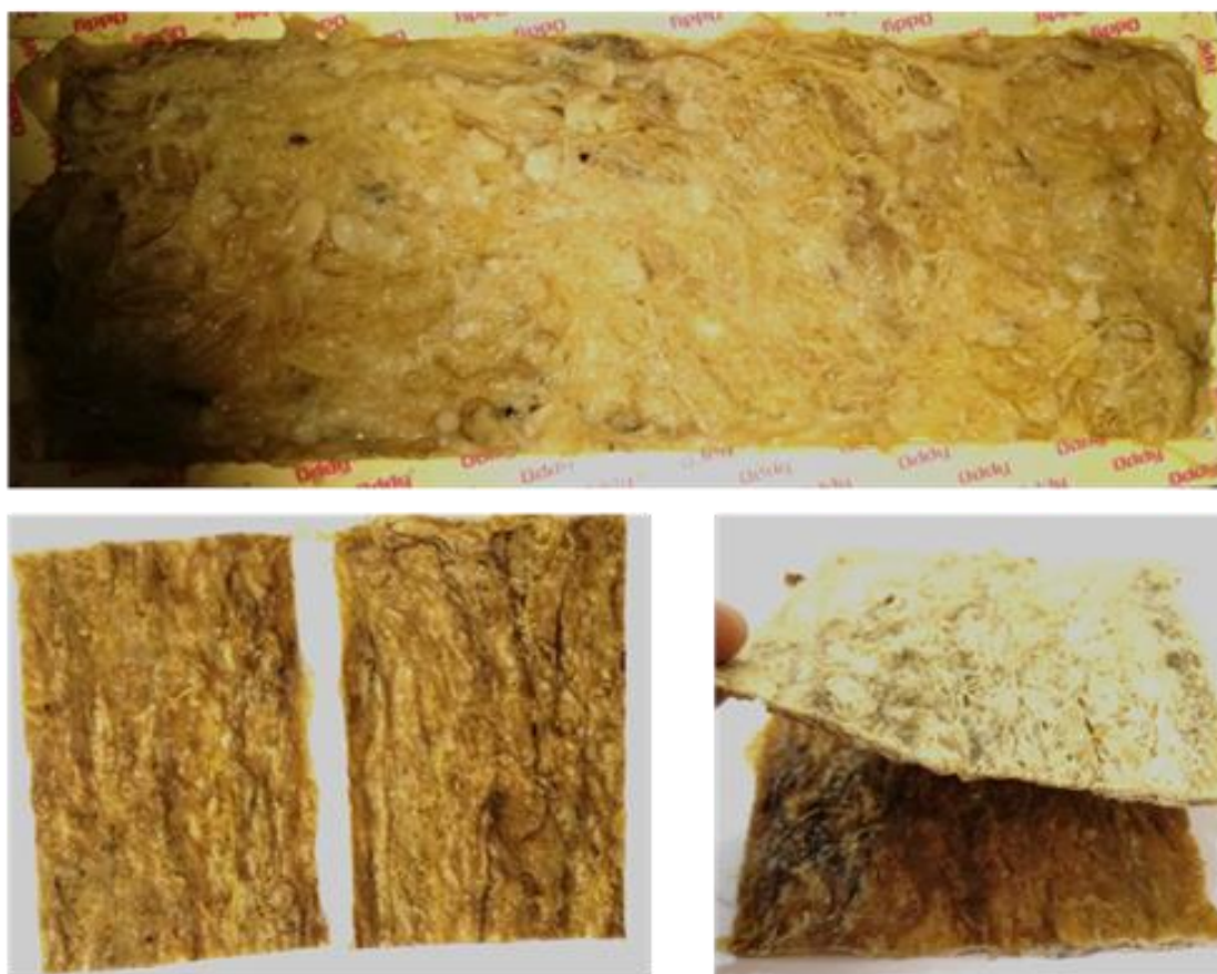
Figure 3.3. Synthesised composite sheets of wheat gluten (WG) and waste Kibisu silk (WKS) with glycerol as plasticiser.
