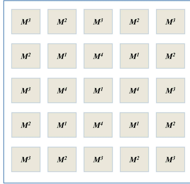
Figure 6.5: Four types of modules are arranged in electrochromic modular architecture.
