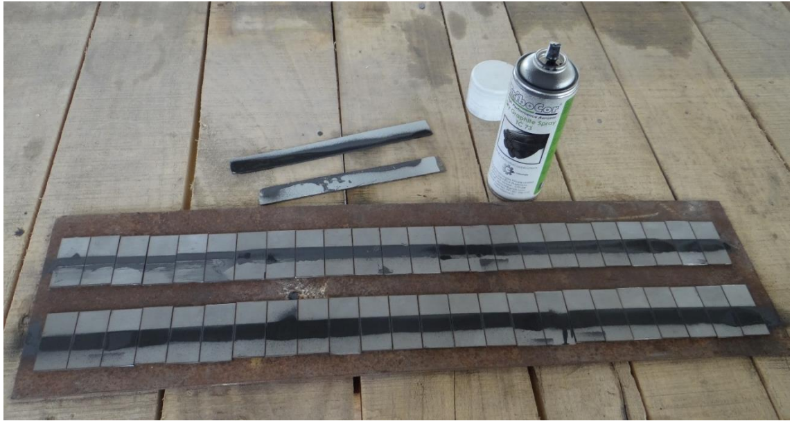
Figure 4-2. Graphite coated duplex-2205 sheet specimens
