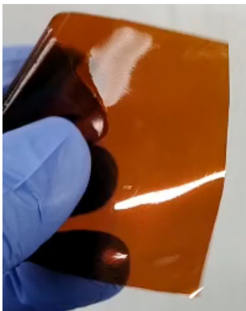
FIGURE 4.2: Picture of the synthesized SPI membrane
