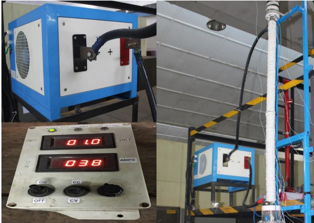
Figure 4.10 Direct Current (DC) power source with its connections and the control unit
