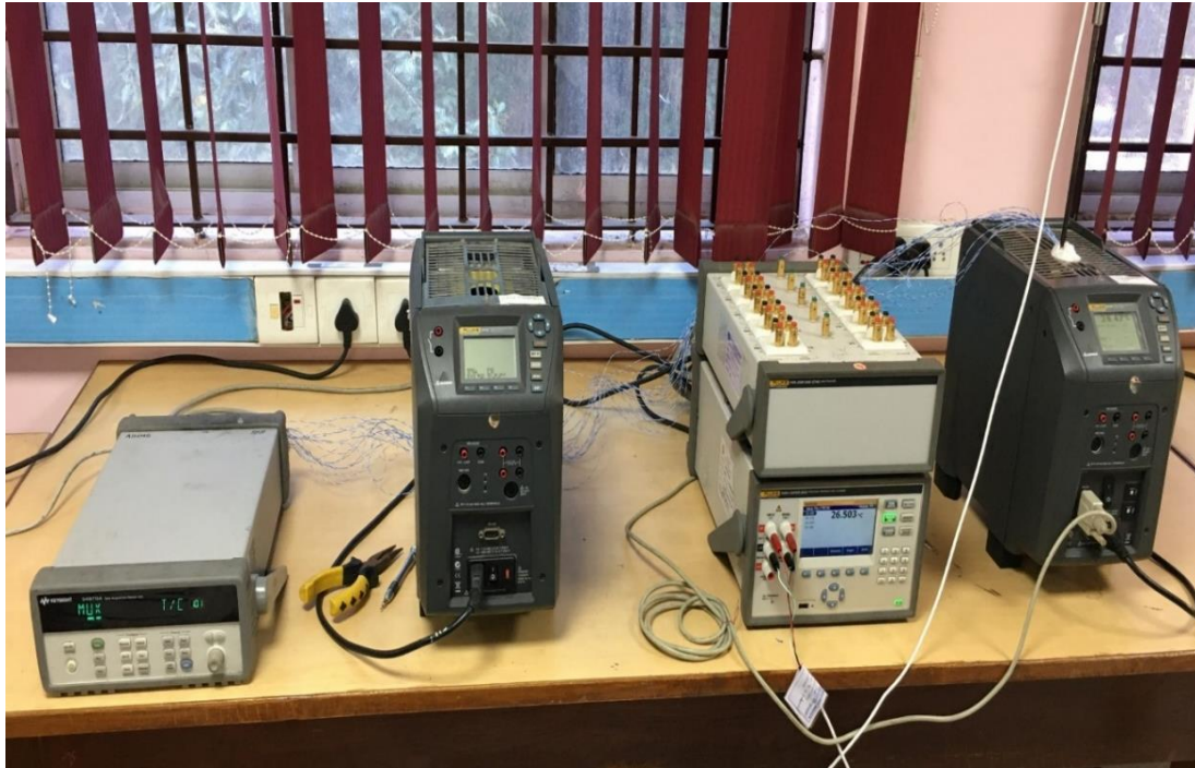
Figure B.1: Calibration of T-type thermocouples and PT 100
