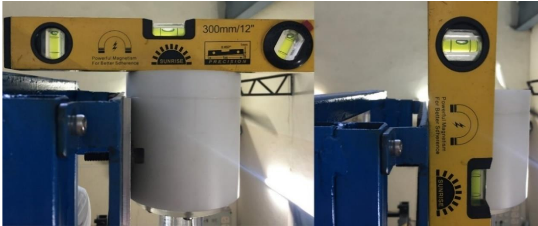
Figure B.4: Vertical and horizontal alignment of the experimental test-rig
