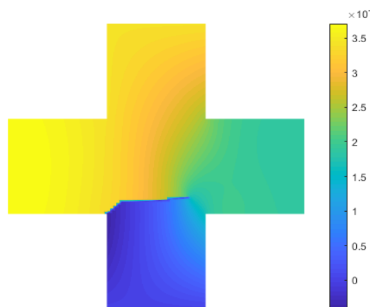
Figure 6.4: Cruciform plate displacement contour (displacement in m) under pure mechanical loading conditions.
