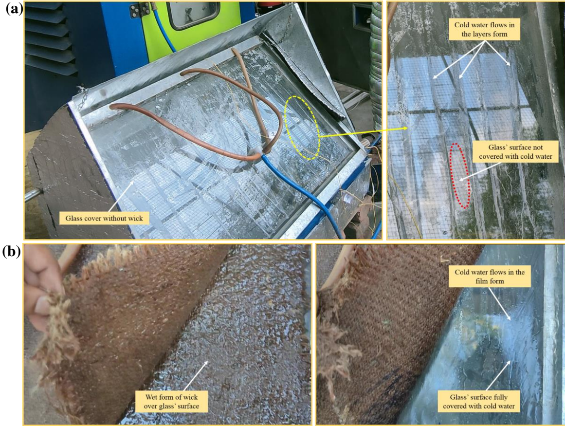
Figure 5.1.8: (a) Structure of cold water flow over glass' surface without wick and (b) effects of wick on m_d through condensation of water vapours
