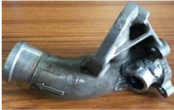
Figure 3.3. Modified intake manifold of the engine for conducting RCCI experiments
