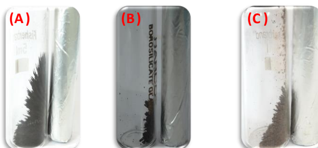
Figure 3b.10. Magnetically separation of A) Fe 3 O 4 , B) IL1@Fe 3 O 4 , and C) IL2@Fe 3 O 4 .
