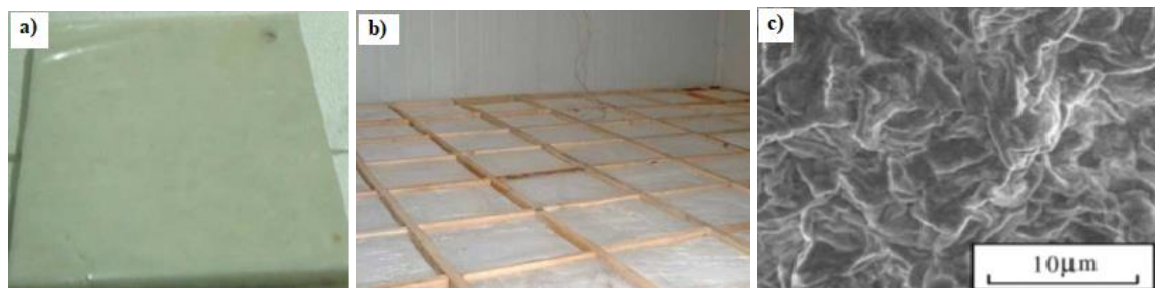
Fig. 2.20 Pictures of SSPCM plate: (a) Plate appearance; (b) SSPCM plate; (c) SEM picture of SSPCM (K. Lin et al., 2005; Y. P. Zhang et al., 2006).
