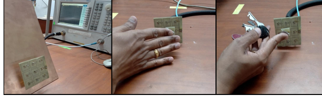
Figure 5.15: Experimental setup with different metallic objects (a) Conducting sheet, (b) Ring, (c) Keychain.
