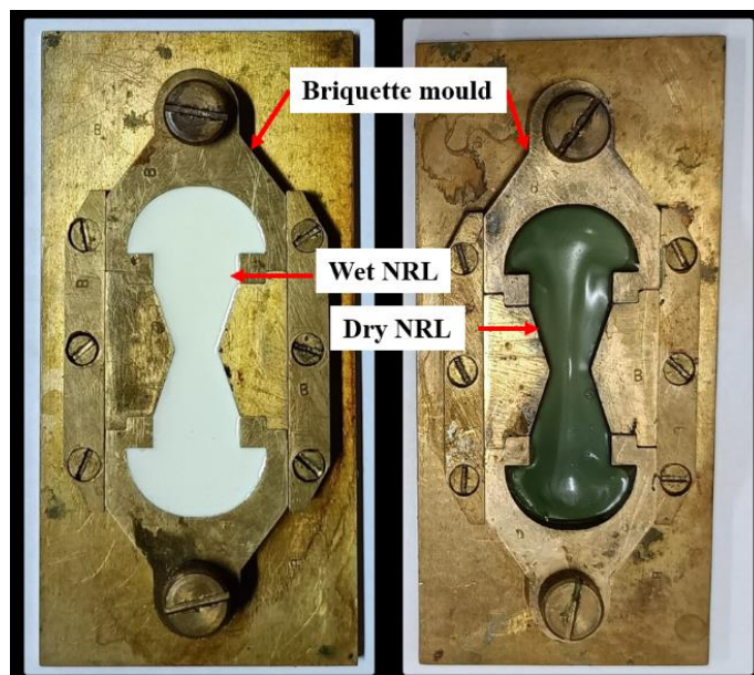
Figure 9. 4 Typical view of dry and wet NRL specimen in briquette mould for ductility test
