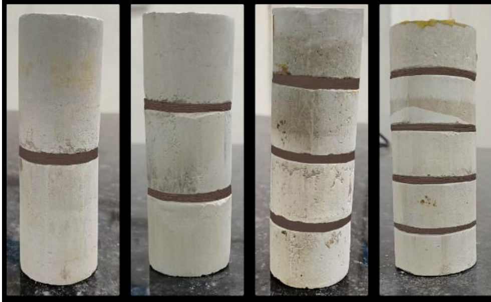
Figure 9. 6 Typical view of plain jointed and NRL grouted jointed Gypsum plaster specimens
