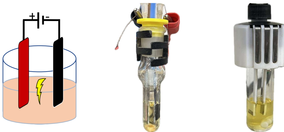
Figure. 1.5.1. Undivided cell setup. Left: schematic representation; Middle: home-made; Right: commercially available Electrasyn 2.0 from IKA.
