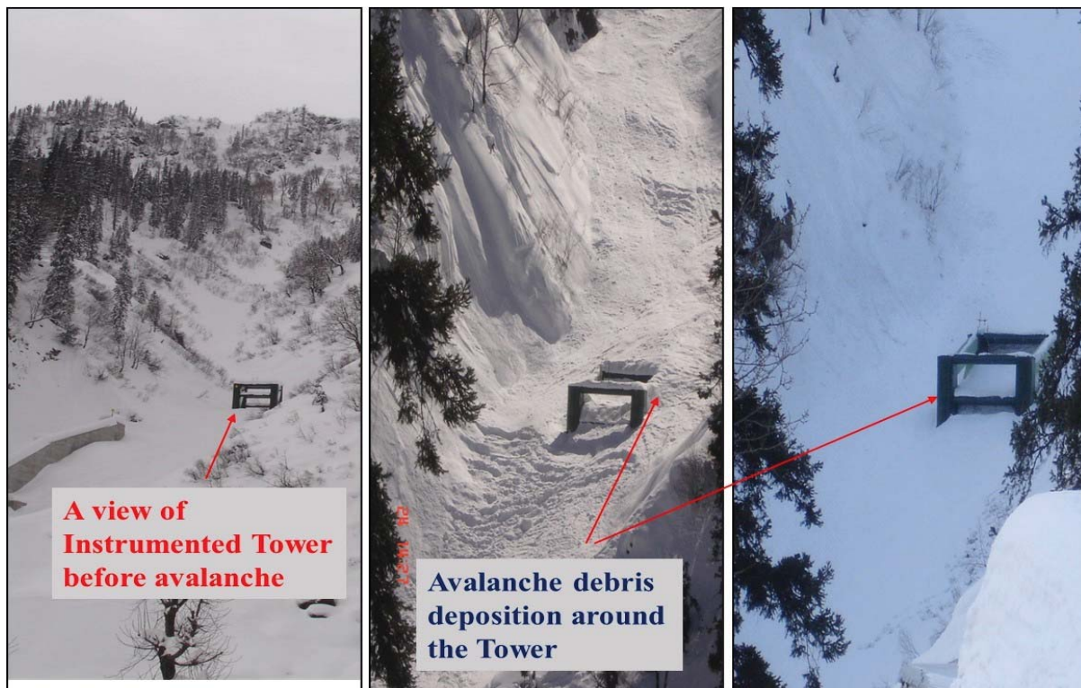
Figure 5.11: Observations of snow deposition around the Instrumented Tower at MSP-10 avalanche site, Dhundhi, Himachal Pradesh, India during the winter period, just before the avalanche occurrence and after the avalanche occurrence
