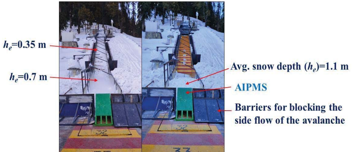
Figure 3.26: Measurement of the avalanche impact pressures P_m by AIPMS after complete blocking of the avalanche flow from the sides with barriers (Experiment E2 on 15 March, 2021)
