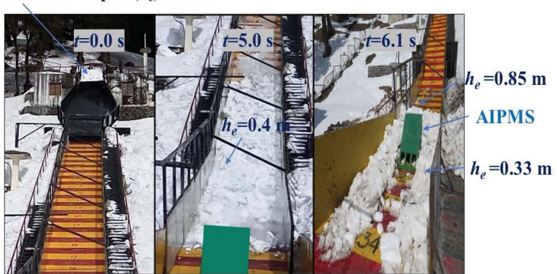
Figure 3.29: Observation of the avalanche flow and its depth at the significant points on the snow chute at various flow time-steps t during the experiment carried out on 17 Feb, 2020
