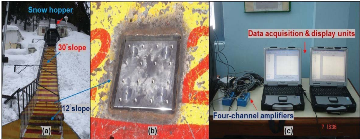
Figure 4.2: (a) A view of the snow chute at Dhundhi, Himachal Pradesh, India (b) close view of the dynamometer installed on 12° slope of the snow chute (c) a view of the data acquisition and display details of the snow dynamic coefficient of friction \mu_k measurement system
