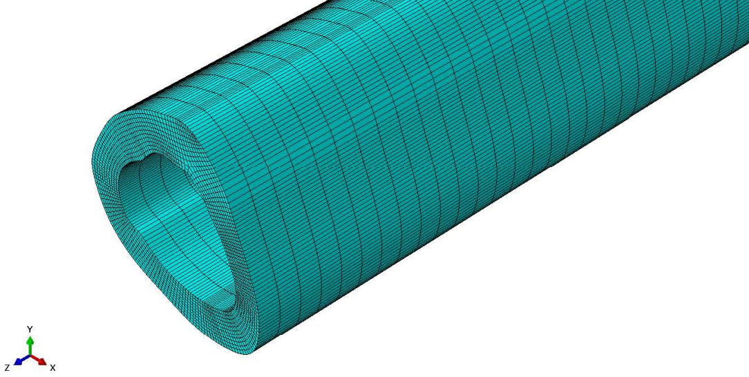
Figure 5.2 The finite element meshed beam has a cross-section similar to the midsection of the mouse tibia.
