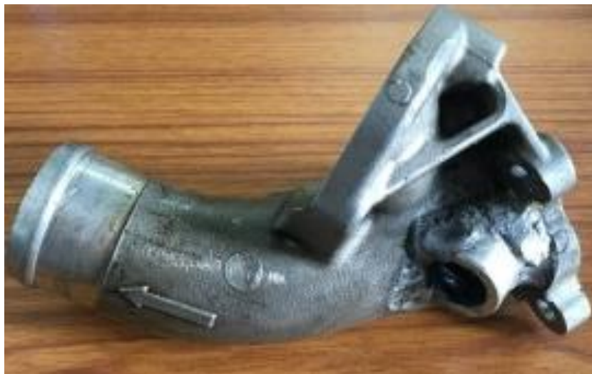
Figure 3.2: Modified intake manifold of the engine for conducting RCCI experiments.
