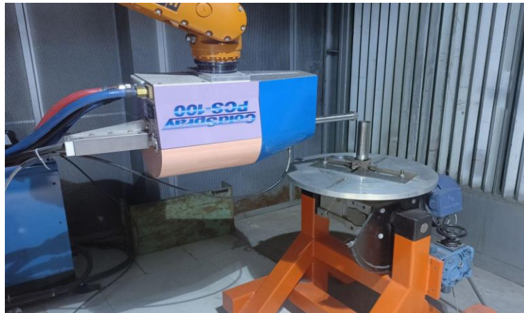
Figure 3.15 Real-time image showing the fabrication of IN 718 thick pipe deposits in progress
