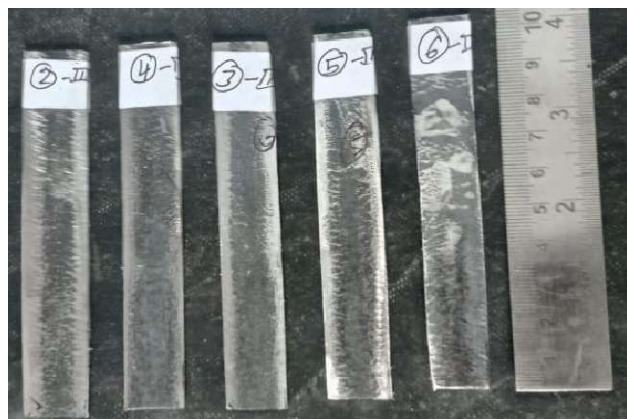
Figure 6.2 The finger-shaped sample is hot rolled to manufacture a sheet, 15 mm wide, and 1.6 mm thick.
