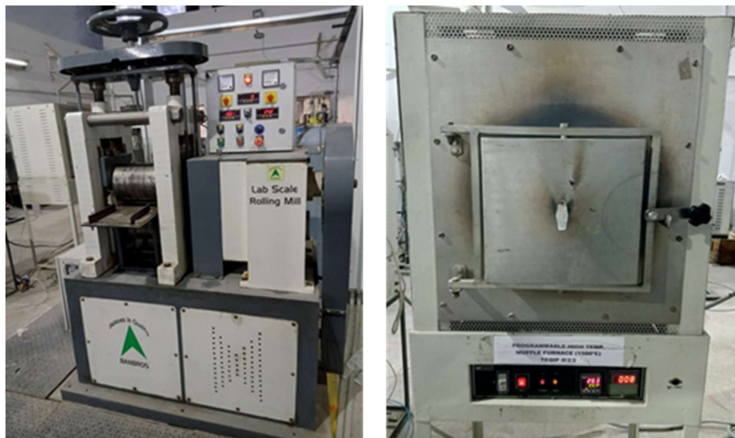
Figure 3.3 Lab scale rolling mill and muffle furnace for thermomechanical treatment
