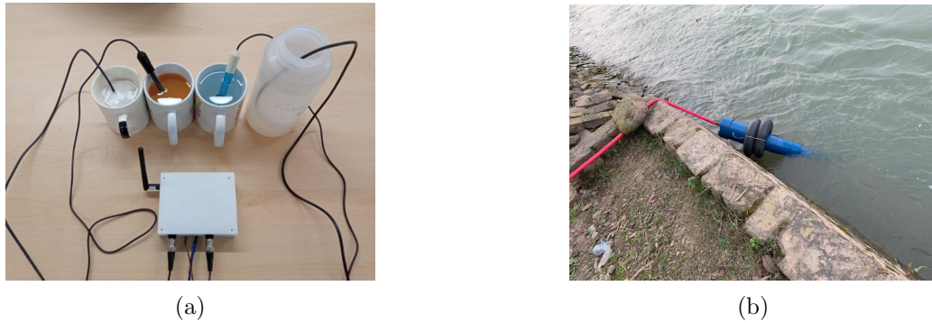
Figure 5.9: Experimental setup of for sensed data accuracy evaluation: (a) design validation and testing with different solutions, (b) setup for river water sensing.
