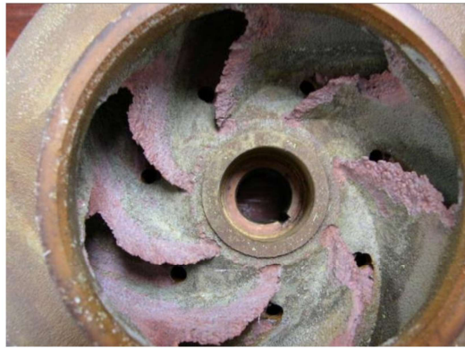
Figure 1.10 Erosion-corrosion of pump impellers [5].
