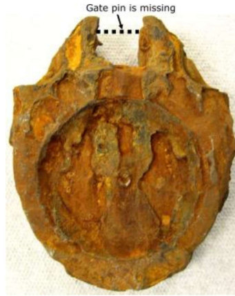
Figure 1.2 Uniform corrosion of a gate valve [5].
