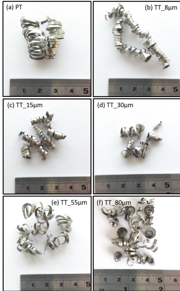
Figure 4.12. Chips obtained during machining operation using plain and textured tools
