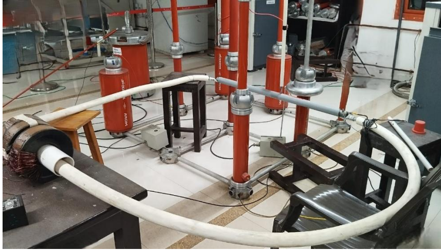
Figure 5.2 Experimental setup for electrical tracking phenomena under varying loading conditions.
