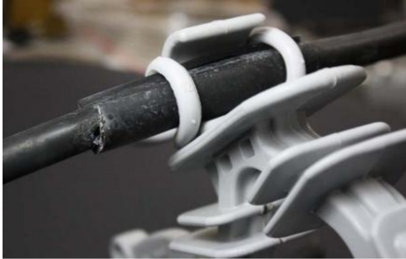
Figure 2.2 Semiconducting tube placed on CC to investigate tracking [13]
