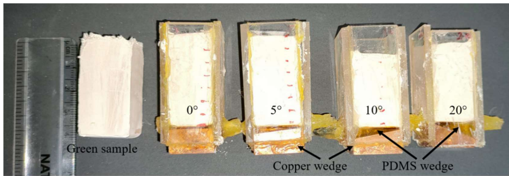
Fig. 2.5 Fabricated green samples with different types of PDMS-copper wedge molds.
