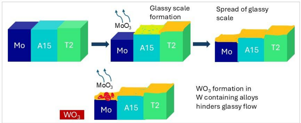
Figure 5.12 Effect of W addition on glassy oxide flow formed during oxidation of Mo-Si-B alloys
