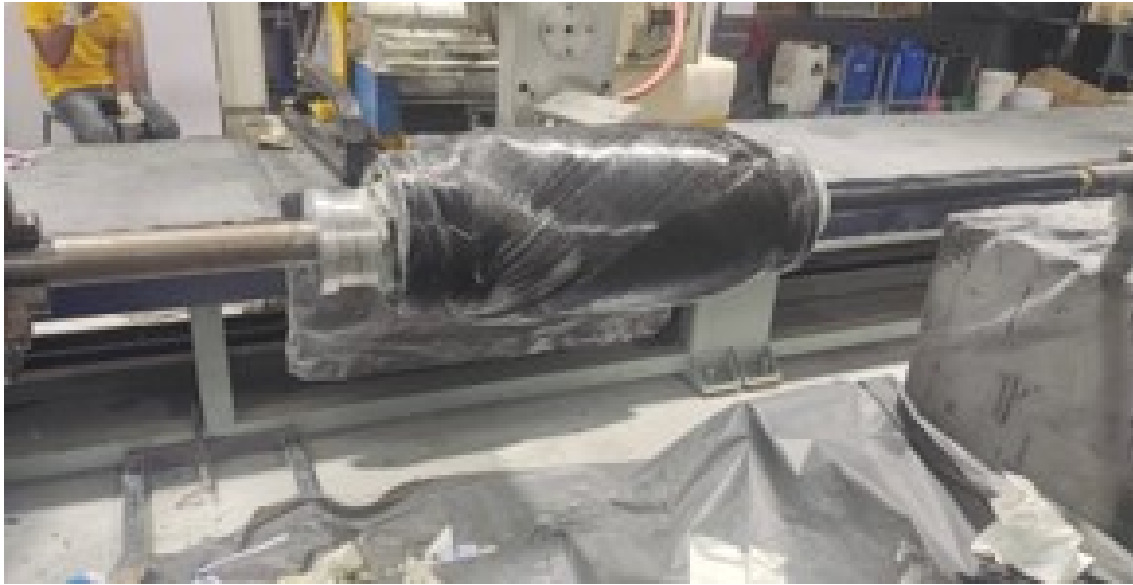
Figure 1.6: Winding of CFRP on the liner-boss assembly during FW process.
