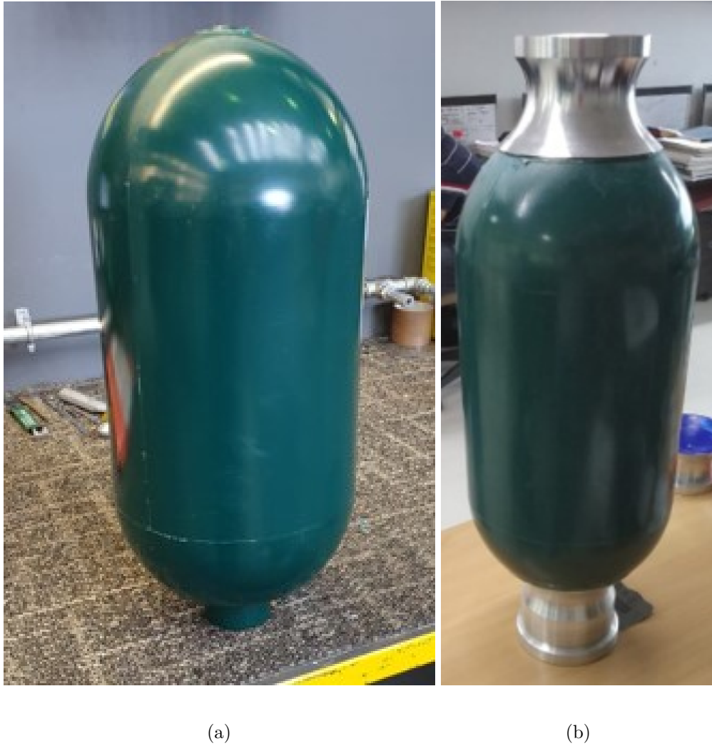
Figure 1.5: (a) Polymer liner procured from Crompton Mouldings, U.K., and (b) liner-boss assembly fabricated at IIT Ropar.
