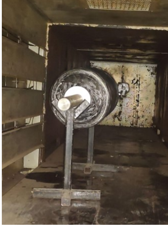
Figure 1.7: Curing of fabricated composite cylinder after wrapping to cure the epoxy resin.
