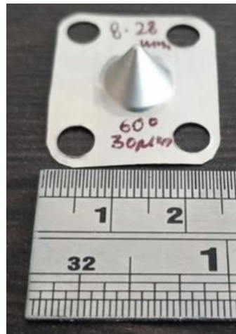
Fig. 6.14: Formed conical geometry through \mu ISF
