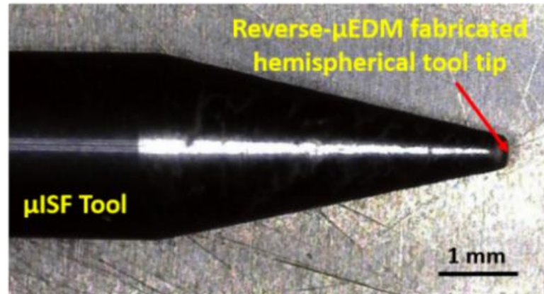
Fig. 6.12: Optical micrograph of the Reverse- \mu EDM fabricated \mu ISF tool
